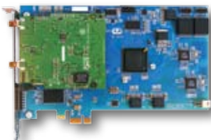
As shown with Epiq Solutions' Bitshark FMC-1RX RF receiver
