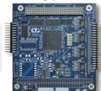
32 single ended/16 differential channels of 16/12 bit analog input, 16 bit GPIO
