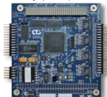
32 single ended/16 differential channels of 16 bit analog input, 4 channels 16 bit analog output, 16 bit GPIO
